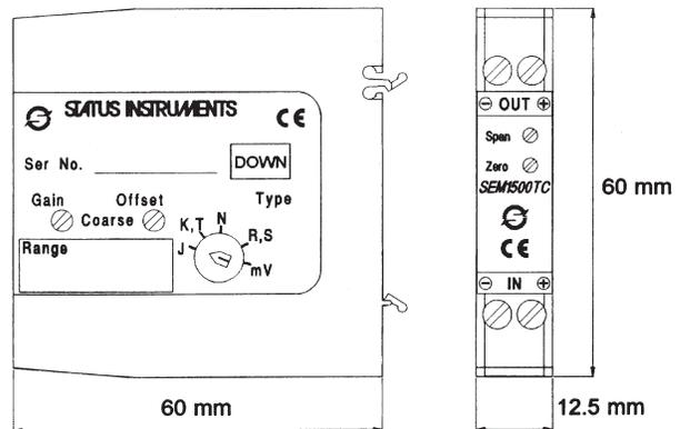
NB. If word "DOWN" appears where shown in label text box then unit has been factory set in the "Down Scale" option, whereas if text box has been left blank then "Up Scale" option has been set.
